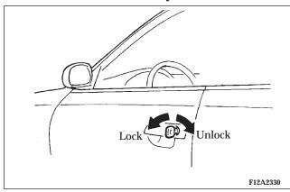
Rotate the key toward the front of the vehicle to lock the door. After checking that the door is locked, turn the key back to the center and remove it from the lock cylinder.
